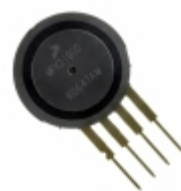
MPX10D NXP USA Inc. SENSOR DIFF PRESS 1.45PSI MAX
