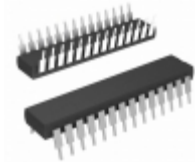
PIC18F26K20-I/SP Microchip Technology IC MCU 8BIT 64KB FLASH 28SDIP
