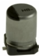
EEV-HB1HR10R Panasonic Electronic Components CAP ALUM 0.1UF 20% 50V SMD
