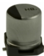
EEV-HB1V100R Panasonic Electronic Components CAP ALUM 10UF 20% 35V SMD
