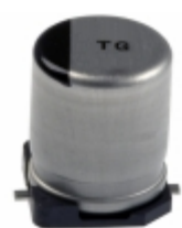
EEV-TG1A331UP Panasonic Electronic Components CAP ALUM 330UF 20% 10V SMD
