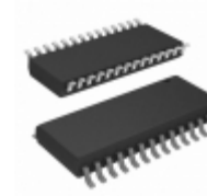
AT28HC256F-12SI Microchip Technology IC EEPROM 256KBIT 120NS 28SOIC
