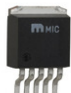
MIC39151-1.65WU-TR Microchip Technology IC REG LDO 1.65V 1.5A TO263-5
