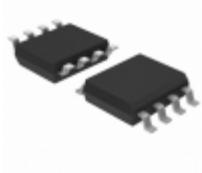
IXG611S1T/R IXYS IC DRIVER MOSF/IGBT 0.6A 8-SOIC
