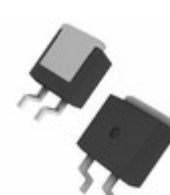
IXGA120N30TC IXYS IGBT 300V 120A 250W TO263AA
