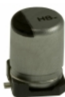
EEV-HB1C100R Panasonic Electronic Components CAP ALUM 10UF 20% 16V SMD
