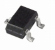
ADM803LAKSZ-REEL7 Analog Devices Inc. IC SUPERVISOR MPU 4.63V SC70-3
