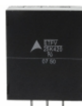
ETFV25K420E4 EPCOS (TDK) VARISTOR 680V 20KA RADIAL
