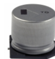
EEV-TG1H102M Panasonic Electronic Components CAP ALUM 1000UF 20% 50V SMD
