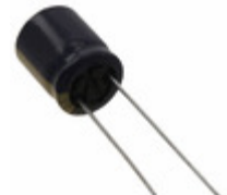
EEU-FC1H331L Panasonic Electronic Components CAP ALUM 330UF 20% 50V RADIAL
