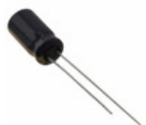
EEU-FC1H390 Panasonic Electronic Components CAP ALUM 39UF 20% 50V RADIAL
