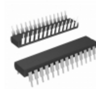
PIC16C62B-04/SP Microchip Technology IC MCU 8BIT 3.5KB OTP 28SDIP
