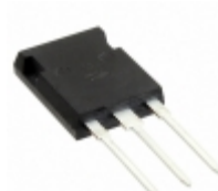
APT34F60BG Microsemi Corporation MOSFET N-CH 600V 34A TO-247
