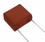
ECW-FA2J474J5 Panasonic Electronic Components CAP FILM 0.47UF 5% 630VDC RADIAL
