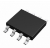
BD9102FVM-TR Rohm Semiconductor IC REG BCK 1.24V 0.8A SYNC 8MSOP
