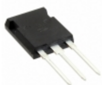
APT34F60B Microsemi Corporation MOSFET N-CH 600V 34A TO-247
