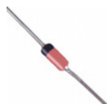
1N5254B-T Diodes Incorporated DIODE ZENER 27V 500MW DO35
