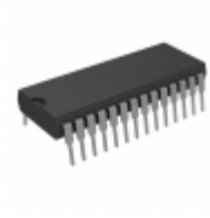
AT28C17E-15PI Microchip Technology IC EEPROM 16KBIT 150NS 28DIP
