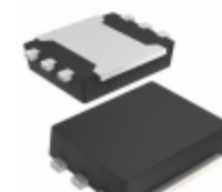
S-1135C17-A6T1U SII Semiconductor Corporation IC REG LINEAR 1.7V 0.3A HSNT-6A
