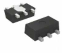
S-1135C17-U5T1G SII Semiconductor Corporation IC REG LINEAR 1.7V 0.3A SOT89-5
