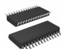
PIC18F26J11-I/SO Microchip Technology IC MCU 8BIT 64KB FLASH 28SOIC
