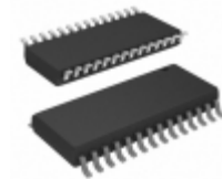
PIC18F2685-E/SO Microchip Technology IC MCU 8BIT 96KB FLASH 28SOIC
