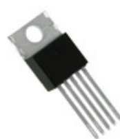
MCP1826-0802E/AT Microchip Technology IC REG LDO 0.8V 1A TO220-5
