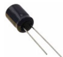
EEU-FC2A390LB Panasonic Electronic Components CAP ALUM 39UF 20% 100V RADIAL
