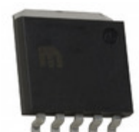
MIC49150-0.9BR Microchip Technology IC REG LDO 0.9V 1.5A SPAK-5
