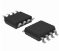
MCP4152-103E/SN Microchip Technology IC POT DGTL SNGL 10K RHEO 8SOIC
