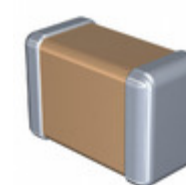
C1206C104K1REC7210 KEMET CAP CER 1206 0.1UF 100V X7R
