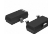
SI2301-TP Micro Commercial Co MOSFET P-CH 20V 2.8A SOT-23
