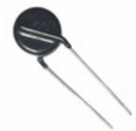
ERZ-E10A511CS Panasonic Electronic Components VARISTOR 510V 4.5KA DISC 11.5MM
