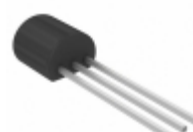
S-80839CLY-Z2-U SII Semiconductor Corporation IC VOLT DETECTOR 3.9V TO-92
