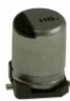
EEE-HBV470YAP Panasonic Electronic Components CAP ALUM 47UF 20% 35V SMD
