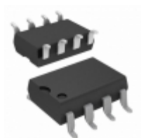
FSQ0365RL Fairchild/ON Semiconductor IC SWIT PWM GREEN OVP UVLO 8SOP
