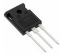
IXFH52N30P IXYS MOSFET N-CH 300V 52A TO-247
