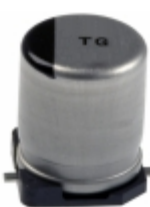
EEV-TG1H470UP Panasonic Electronic Components CAP ALUM 47UF 20% 50V SMD
