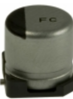
EEV-FC1V100R Panasonic Electronic Components CAP ALUM 10UF 20% 35V SMD
