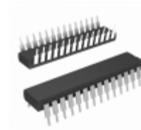
PIC24FJ32MC102-E/SP Microchip Technology IC MCU 16BIT 32KB FLASH 28SDIP
