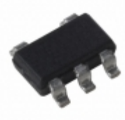
MIC5247-1.85BM5-TR Microchip Technology IC REG LDO 1.85V 0.15A SOT23-5
