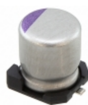
10SVP33M Panasonic Electronic Components CAP ALUM POLY 33UF 20% 10V SMD
