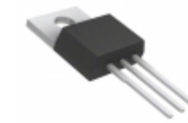
TIP49 AMI Semiconductor / ON Semiconductor TRANS NPN 350V 1A TO-220
