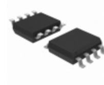
AT93C66AW-10SI-1.8 Microchip Technology IC EEPROM 4KBIT 2MHZ 8SOIC
