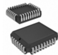
AT28C64X-15JC Microchip Technology IC EEPROM 64KBIT 150NS 32PLCC
