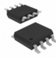
AO4454 Alpha & Omega Semiconductor Inc. MOSFET N-CH 100V 6.5A 8SOIC
