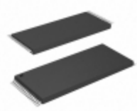
AT27C080-90TI Microchip Technology IC OTP 8MBIT 90NS 32TSOP
