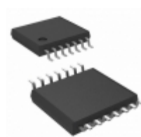
MC74VHCT14ADR2G ON Semiconductor IC INVERT HEX SCHMT CMOS 14TSSOP
