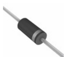
BZW06-299 R0G TSC (Taiwan Semiconductor) TVS DIODE 299V 618V DO204AC
