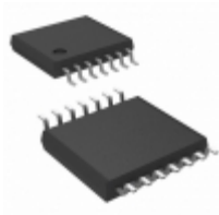
AD5207BRUZ10 Analog Devices Inc. IC DGTL POT DUAL 10K 14-TSSOP
