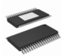
LTC3859AMPFE#TRPBF ADI (Analog Devices, Inc.) IC REG CTRLR MULT TOP 38TSSOP
