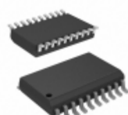
PIC16LF1508-E/SO Microchip Technology IC MCU 8BIT 7KB FLASH 20SOIC
