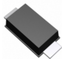
KDZVTR4.3B Rohm Semiconductor DIODE ZENER 4.3V 1W PMDU
