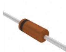
1N5256B A0G TSC (Taiwan Semiconductor) DIODE ZENER 30V 500MW DO35
