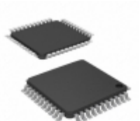
PIC32MX270F256DT-50I/PT Microchip Technology IC MCU 32BIT 256KB FLASH 44TQFP
